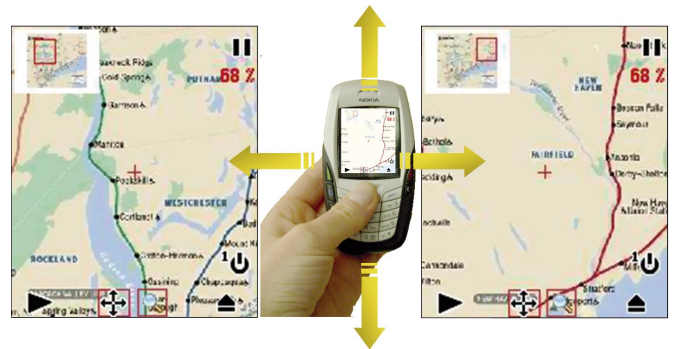
Moving the camera left, right, up, or down moves the image to the desired area of interest
